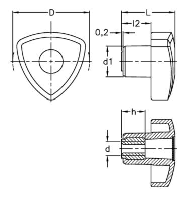
$$\begin{array}{ll} d & = 32 \\ d1 & = 14 \\ d \ 6H = M6 \\ L & = 26 \\ l2 & = 16 \end{array}$$
